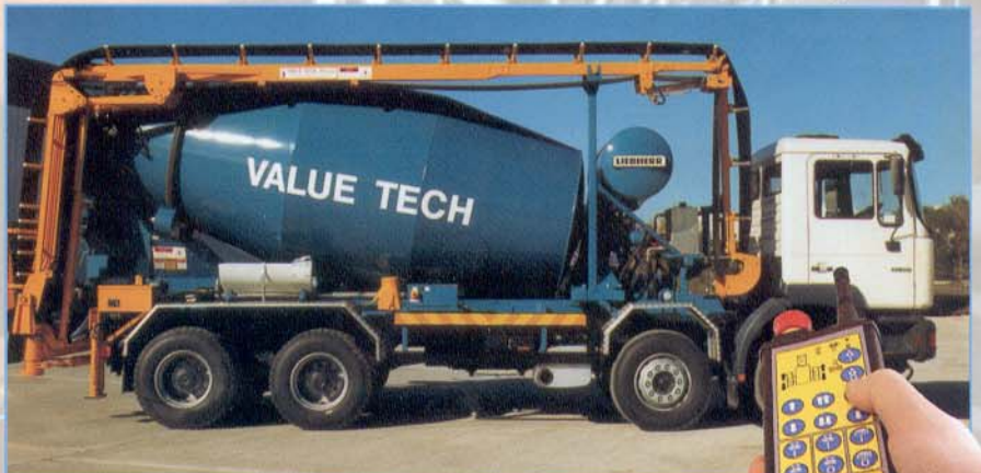
Concrete Mixer and Conveyor Control
